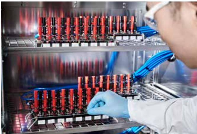
A BASF scientist in Shanghai works with small test batteries, which can provide precise data on battery lifetime performance for electric vehicles.
